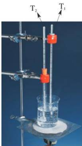
Fig. 8 Melting of mothball flakes. Thermometer ( T_1 ) reads the temperature of mothball flakes, and thermometer ( T_2 ) reads the temperature of the water bath.
