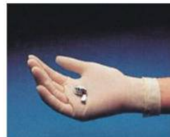
Fig. 23 The melting point of gallium is 29.8°C. Body temperature is 37°C, which is enough to cause the metal to melt in the palm of your hand.
