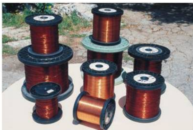
Fig. 22 Metals can be drawn into wires. The gauge of the wire is related to its thickness.
