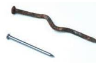
Fig. 35 Rusted iron. The formation of rust weakens the metal.
