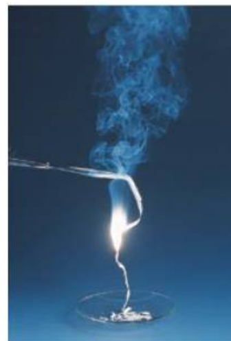
Fig. 6 Magnesium burns with a brilliant flame. Magnesium oxide (white powder) is the product of the reaction.
