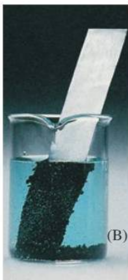
Fig. 28b Copper metal atoms are deposited on the zinc strip. Almost, the reaction is complete.
