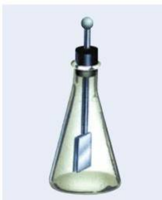
Fig. 25b An electroscope is a device which detects static electric charges.
