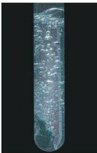
Fig. 16 The reaction of zinc with hydrochloric acid produces hydrogen gas bubbles.
