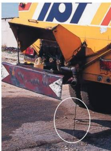
Fig. 33 Ground wire on a fuel truck.
