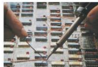
Fig. 30 Solder (an alloy of lead and tin) can be melted with a hot iron to join electrical components without damaging them.
