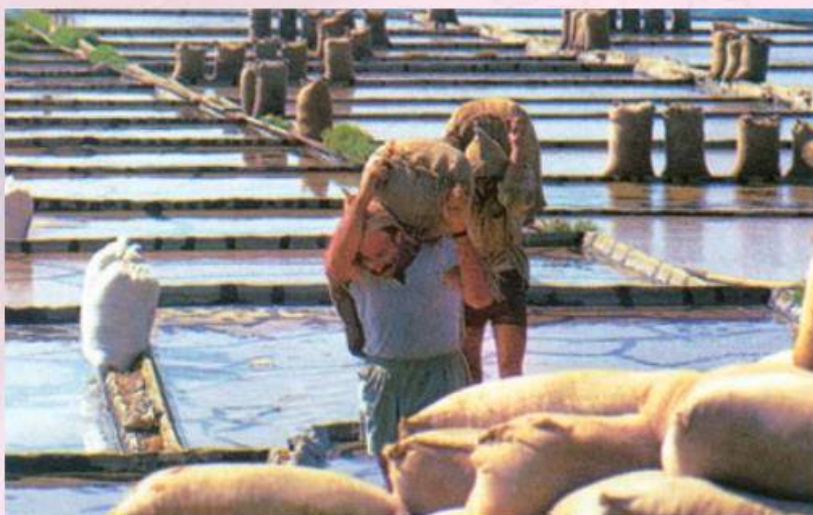
Fig. 2 Seawater is trapped in small ponds, the sun's heat evaporates away the water, leaving behind the salt.
