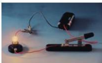
Fig. 16b An electric circuit must form a continuous path in order for electrons to travel.
