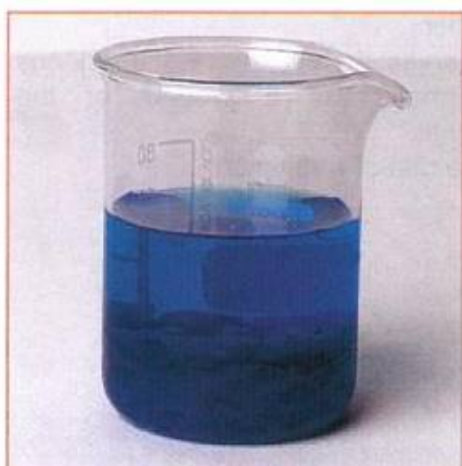
Figure 2.2 The formation of Cu(OH)_2 precipitate is an instantaneous reaction between Cu_{(aq)}^{2+} ions and HO_{(aq)}^- ions.
