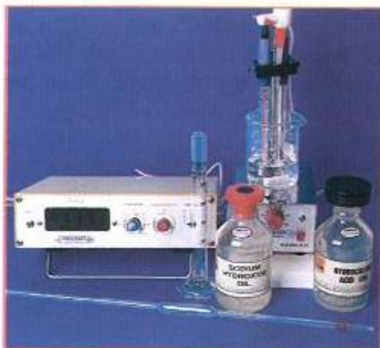
Figure 5.15 Set up for the pH-metric study of an acid-base reaction.
