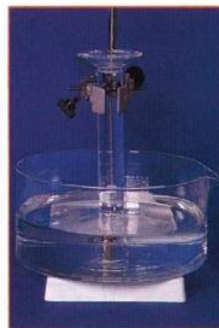
Figure 1.6 Apparatus for measuring the volume of hydrogen released.
